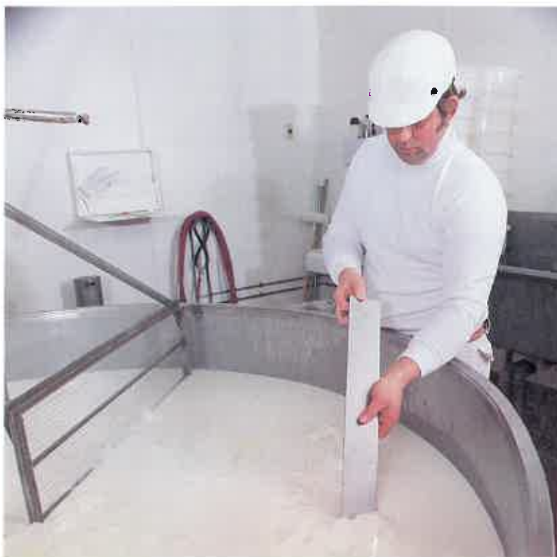
Figure 20.17 ▶ A cheesemaker checks the consistency of milk that has been curdled by rennin.
